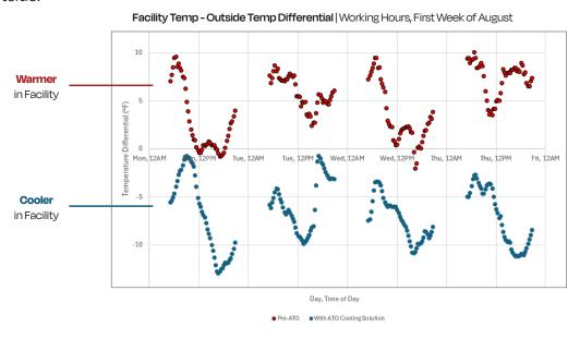
After installing the ApexAir, we saw a clear shift toward consistently negative differentials, showing that the system kept indoor conditions cooler even as outdoor temperatures peaked. Measuring the inside-outside differential allowed us to cut through daily weather swings and get a reliable view of real-world performance.
